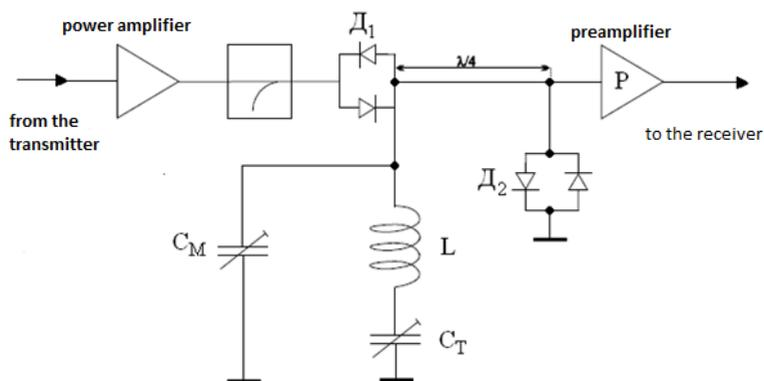
Figure 2. Switching scheme of the NQR signal sensor with the transmitter output and the preamplifier input. Here  $S_M$  is an alternating capacitor for matching the circuit,  $C_T$  is a variable capacitor for tuning the circuit at the resonant frequency,  $D_1$  and  $D_2$  cross-diodes
