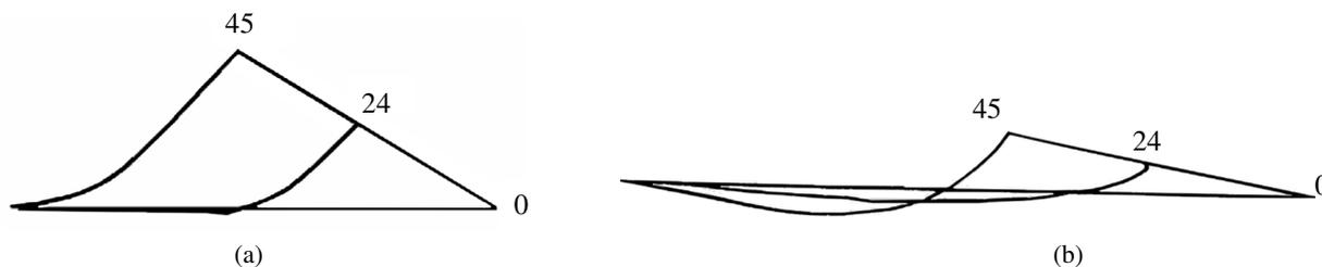
Fig. 6. Shape of the shock absorber in motion: (a)  $m_b = 25$  kg;  $k = 10$ ;  $\alpha = 30^\circ$ ; (b)  $m_b = 25$  kg;  $k = 10$ ;  $\alpha = 10^\circ$ .
