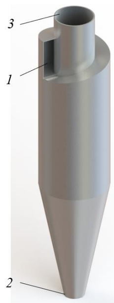
Figure 1. A real-world 3D model of the TsN-15 cyclone: (1) the inlet for the gas contaminated by the catalyst; (2) the outlet for catalyst particles collected during purification; and (3) the outlet for purified gas.
