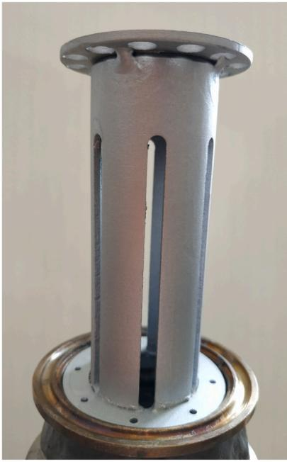
Fig. 6. Photo of the vortex contact device.
