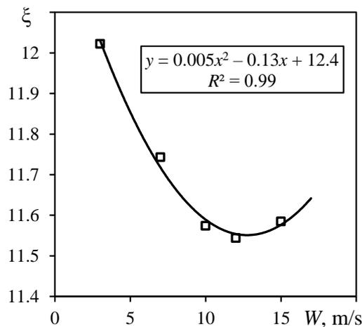
**Figure 5.** Pressure drop coefficient versus the inlet gas velocity.
