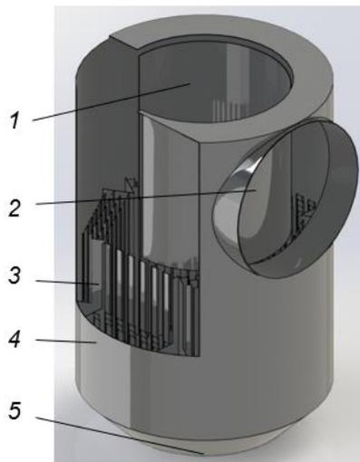
**Figure 1.** Separation device with sections of double-T elements (section view): 1 – inlet pipe; 2 – outlet pipe; 3 – section of double-T elements; 4 – cylindrical body; 5 – outlet pipe for dust bunker.
