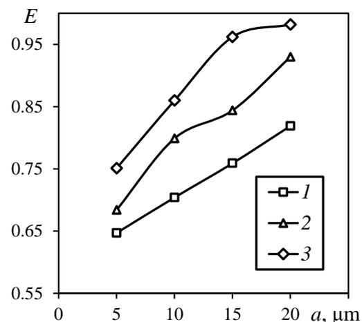
**Figure 4.** Separation efficiency versus particle size at different particle density, kg/m<sup>3</sup>: 1 – 1000; 2 – 3000; 3 – 7000. Inlet gas velocity  $W = 15$  m/s.
