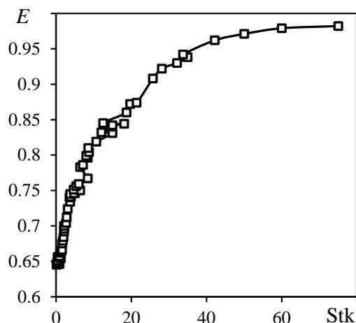
**Figure 3.** Separation efficiency versus Stokes number.
