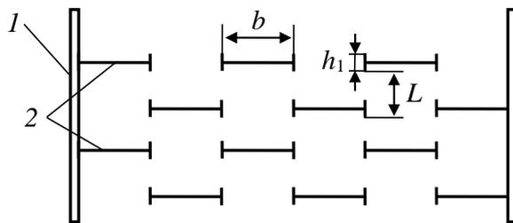
**Figure 2.** Scheme of a section of double-T elements (top view): 1 – section wall; 2 – double-T elements.
