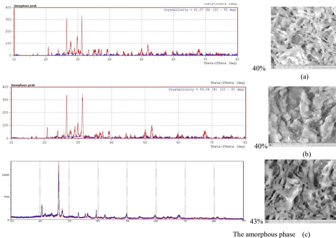
FIGURE 2. X-ray patterns, percentage of amorphous phase and microphotographs of fractures of samples fired in a microwave oven of compositions: (a) - diatomite, marl, NaCl; (b) - marl, NaCl; (c) - diatomite, NaCl.
