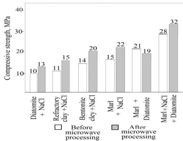
FIGURE 1. Dependence of the strength of the material on the composition of the composition.
