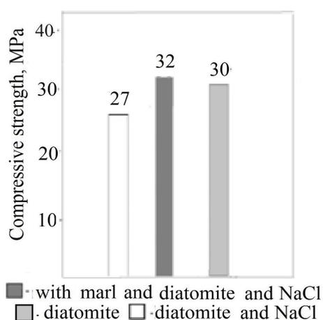
**Figure 2.** Strength of samples based on diatomite with marl and NaCl salt additives after firing at 1000 °C.
