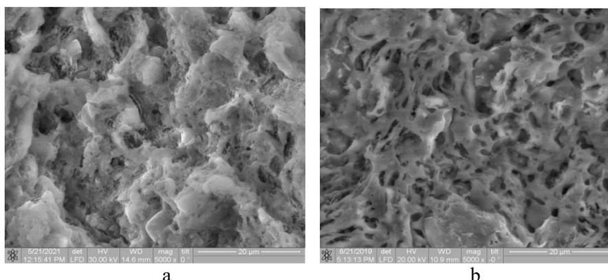
**Figure 3.** Fracture micrographs of samples of burnt diatomite (a) and a mixture of diatomite with marl and NaCl salt (b).
