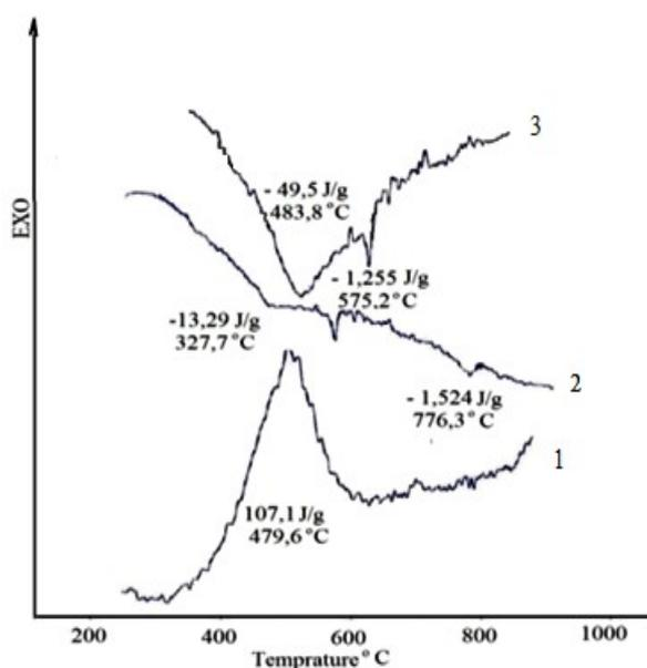
**Figure 1.** Differential and thermal curves of compositions on the basis of diatomite – 1, with NaCl salt inclusion – 2, with inclusions of NaCl and marl – 3.
