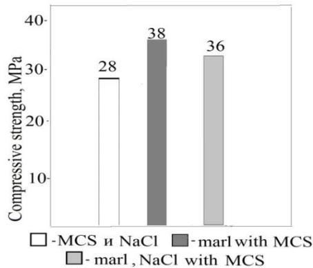
**Fig. 2.** Dependence of the strength of the material on the composition of the composition
