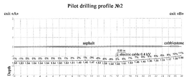
Fig. 9. Pilot drilling profile of paper-insulated cable
