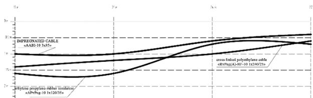
Fig. 13. The depth of the CL along the length in the third part in the section from 18 to 27 meters
