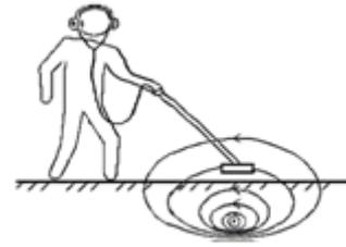
Fig .3. Induced signals in the induction method.
