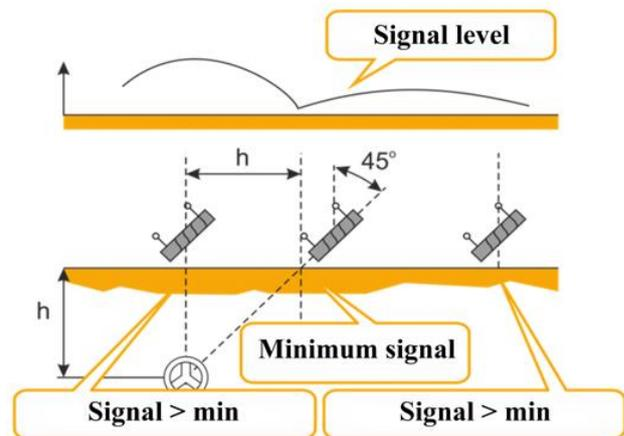
Fig .4. The theoretical explanation of 45 degree method
