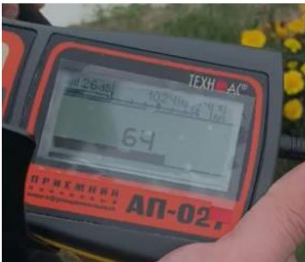
Fig .2. Line locator system receiver
