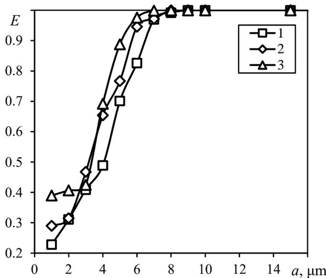
**Figure 5.** Separation efficiency versus particle size under different particle densities  $\rho_a$ ,  $\text{kg/m}^3$ : 1 – 2000; 2 – 2330; 3 – 3000. Inlet gas velocity  $W = 10$  m/s.
