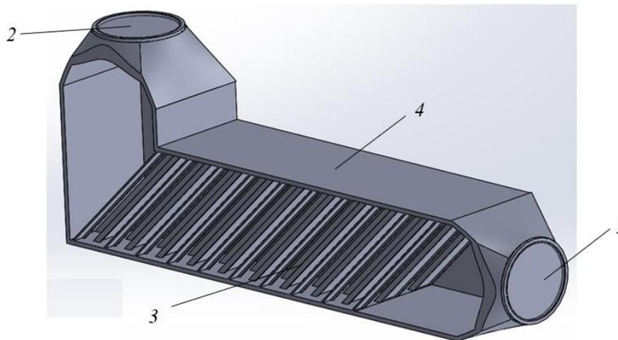
**Figure 1.** Simplified 3D separator model with inclined double-T elements: 1 – inlet; 2 – outlet; 3 – double-T elements; 4 – body.
