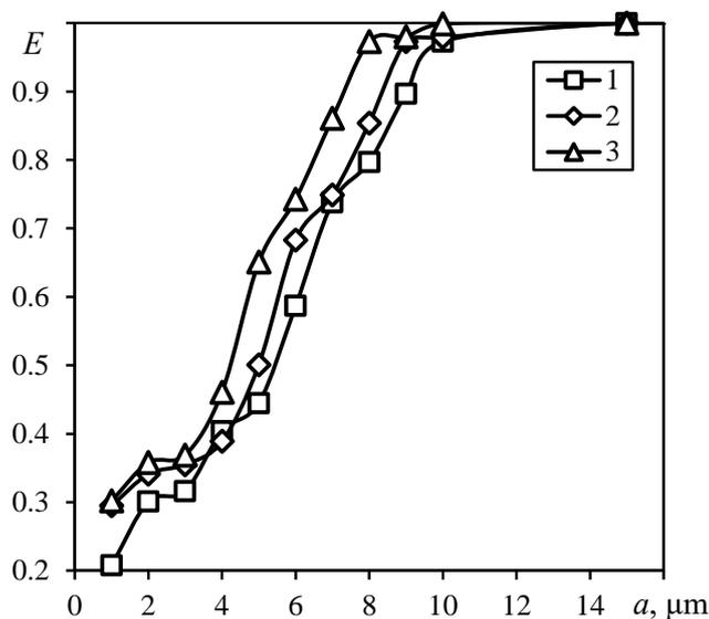
**Figure 3.** Separation efficiency versus particle size under different particle densities  $\rho_a$ ,  $\text{kg/m}^3$ : 1 – 2000; 2 – 2330; 3 – 3000. Inlet gas velocity  $W = 5$  m/s.
