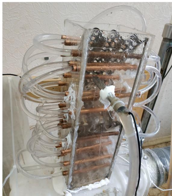
Fig. 4. Real image of fill pack with three-flow cooling circuit.
