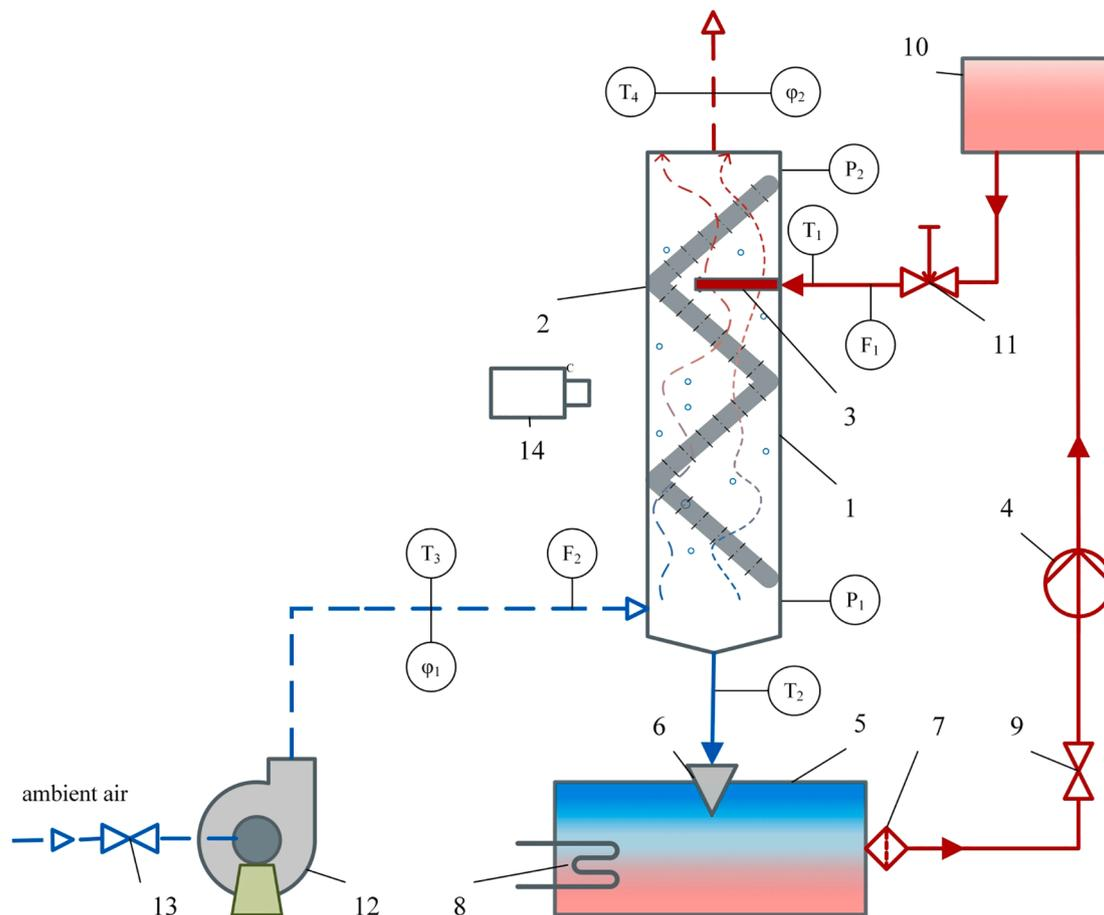
Fig. 2. Schematic diagram of experimental system: 1 – fill pack; 2 – inclined-corrugated contact elements; 3 – water distributor; 4 – pump; 5, 10 – water tank; 6 – funnel; 7 – liquid filter; 8 – heaters; 9, 11 – shutoff valves on the water supply line; 12 – fan; 13 – shutoff valves in the air supply line; 14 – camera.
