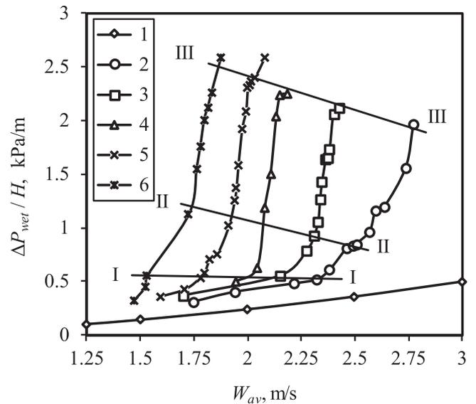
**Fig. 6.** Hydraulic characteristics of wetting fill pack (type 3) at different wetting rates  $q_v$ , m<sup>3</sup>/(m<sup>2</sup>·h): 1 – 0; 2 – 11.8; 3 – 18.0; 4 – 24.3; 5 – 30.6; 6 – 36.8; I-I – loading points; II-II – flooding points; III-III – superflooding points.
