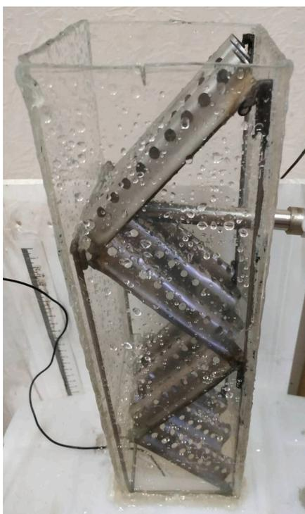
Fig. 1. Real image of fill pack with inclined-corrugated contact elements.
