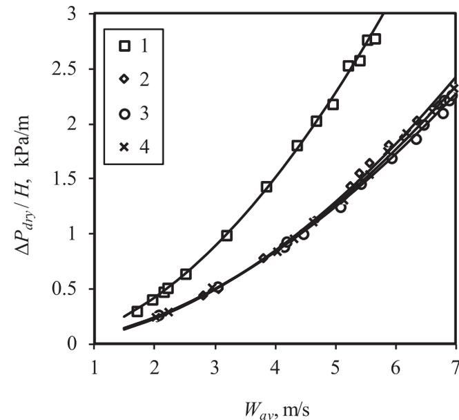
**Fig. 5.** Pressure drop in different types of dry fill packs: 1 – ICCE with 5 mm holes; 2 – ICCE with 6 mm holes; 3 – ICCE with 6 mm holes and metal grid; 4 – with the three-flow cooling circuit; dots – experimental points, solid lines – according to Eq. (1) (Table 2).
