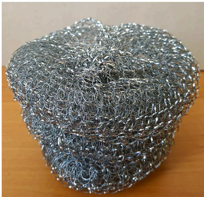
Fig. 3. Real image of metal grid used in fill pack.
