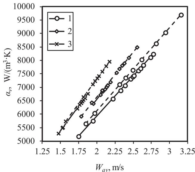
Fig. 11. Volumetric heat transfer coefficient vs. average gas velocity at various wetting rates  $q_m$ ,  $\text{kg}/(\text{m}^2\cdot\text{s})$ : 1 – 3.25; 2 – 6.70; 3 – 10.15; solid lines – type 3 (with metal grid); dashed lines – type 2.
