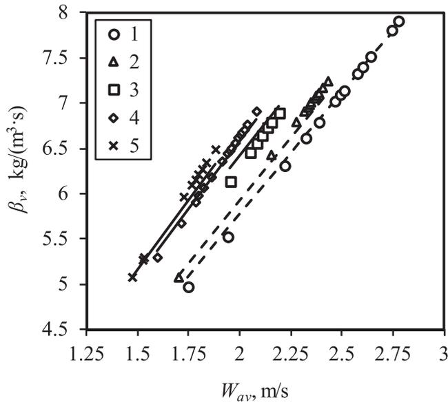
**Fig. 8.** Volumetric mass transfer coefficient vs. average gas velocity for fill pack (type 3) at various wetting rates  $q_m$ ,  $\text{kg}/(\text{m}^2\cdot\text{s})$ : 1 – 3.25; 2 – 4.97; 3 – 6.70; 4 – 8.42; 5 – 10.15; dots – experimental points, dashed lines – according to Eq. (12.1), solid lines – according to Eq. (12.2).
