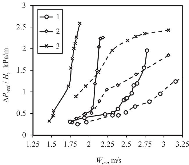
Fig. 7. Pressure drop in wetting fill pack vs. average gas velocity at different wetting rates  $q_v$ ,  $m^3/(m^2 \cdot h)$ : 1 – 11.8; 2 – 24.3; 3 – 36.8; solid lines – type 3 (with metal grid); dashed lines – type 2.
