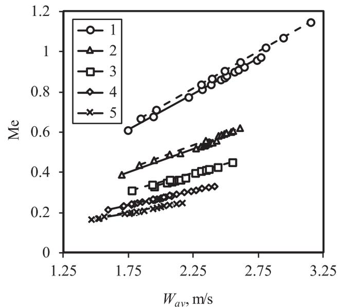
Fig. 12. Variations of Merkel number with average gas velocity at various wetting rates  $q_m$ ,  $\text{kg}/(\text{m}^2\cdot\text{s})$ : 1 – 3.25; 2 – 4.97; 3 – 6.70; 4 – 8.42; 5 – 10.15; solid lines – type 3 (with metal grid); dashed lines – type 2.
