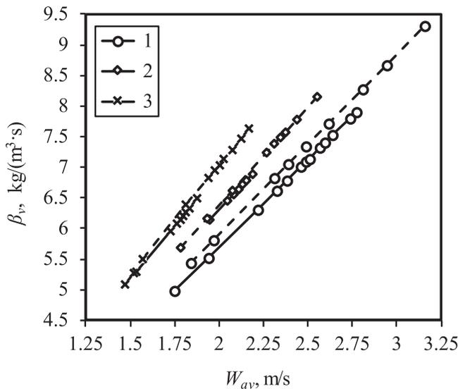
**Fig. 9.** Volumetric mass transfer coefficient vs. average gas velocity at various wetting rates  $q_m$ ,  $\text{kg}/(\text{m}^2\cdot\text{s})$ : 1 – 3.25; 2 – 6.70; 3 – 10.15; solid lines – type 3 (with metal grid); dashed lines – type 2.
