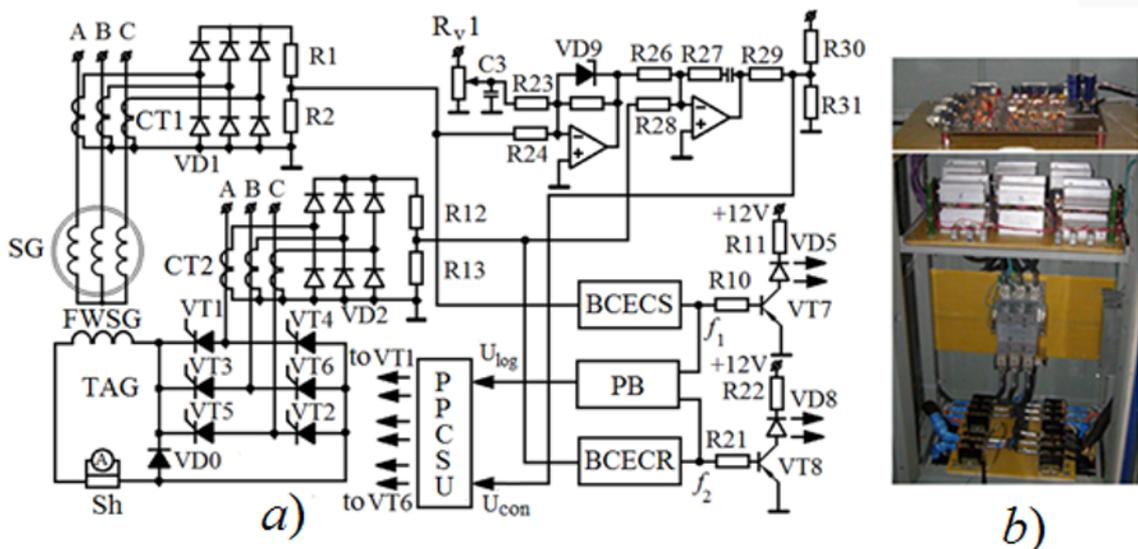
**Fig. 10.** A device for automatically controlling the excitation of a synchronous generator: a) - schematic diagram; b) - control board and power unit.
