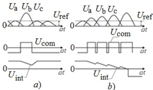
**Fig. 6.** Voltages at various links of the unit for calculating the emergency current of the rotor of the synchronous generator and unit for calculating the emergency current of the synchronous generator circuits.
