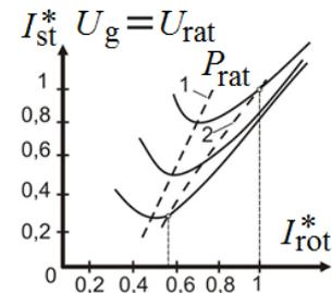
**Fig. 4.** Compounding characteristics of a synchronous generator.
