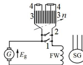
**Fig. 3.** Scheme automatic field suppression type AHL-1 plant "Electrosila".
