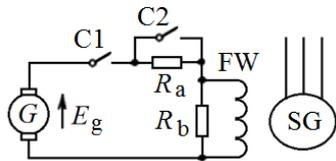
**Fig. 1.** The circuit of the excitation winding of the synchronous generator to the anchor circuit of the generator to a controlled pathogen.
