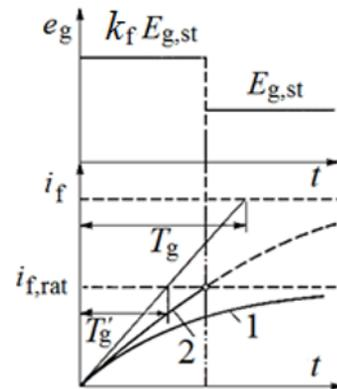
**Fig. 2.** Graphs of variance in the excitation voltage and the electromotive force of the pathogen during startup with forced.
