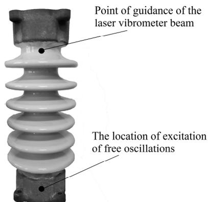
Fig. 6. Point of guidance of the laser vibrometer beam and the location of excitation of free oscillations
