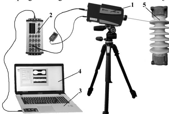
Fig. 2. Diagram of device and measurement of the complex: 1 - Laser Vibrometer PDV-100; 2 - multi-function input-output module (BNC 6212); 3 - personal computer; 4 - software; 5 - object of study
