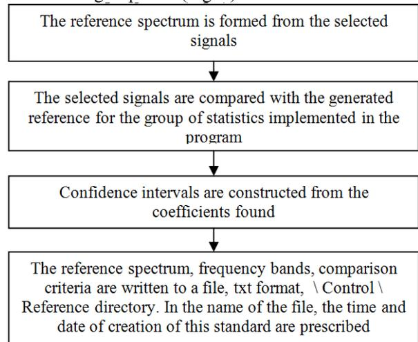
Fig. 4. Sequence of work of the subprogram "Formation of reference spectra".
