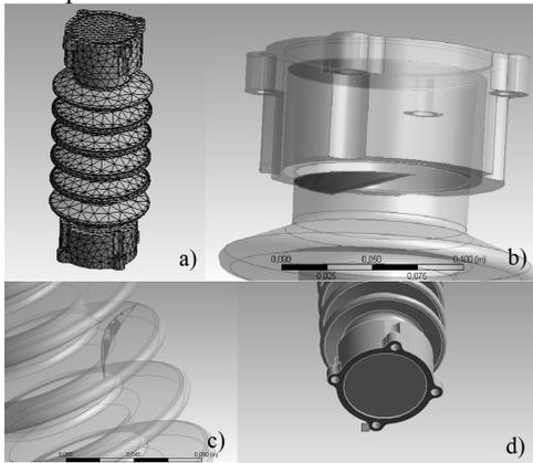
Fig. 1. a – finite-element model of the SRI, b – crack of the insulator's trunk, c – crack of the insulator rib, d – hard seal.
