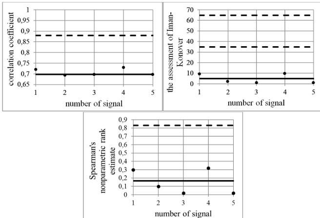
Fig. 7. The results of comparison of the reference (defect-free) and defective (trunk core of the insulator near the upper flange) SRI
