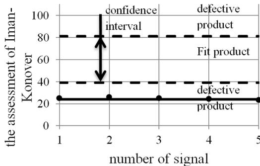
Fig. 3. The principle of constructing the decisive "fit-defective" rule by the example of the Iman-Konover estimate
