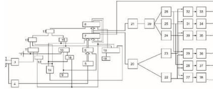
**Fig. 1.** Structural scheme of a metering device that implements the methodology for adjusting the cost of electricity depending on its quality.
