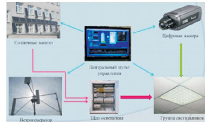
Fig. 3. Block diagram of the demonstration and laboratory complex of the intelligent artificial lighting systems and alternative energy
